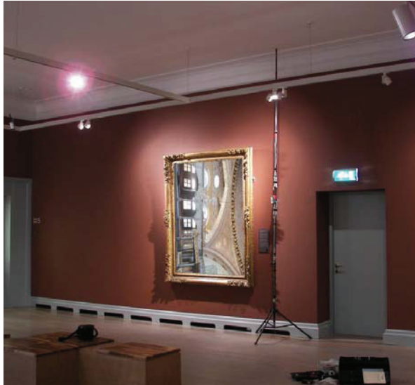
Figure 6. Test set up for measuring temperature stratification at room level.
